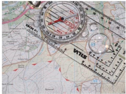
1: Line the base plate of the compass along the line of travel on the map
