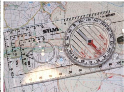
3: Turn the whole compass until the needle sits within the arrow outline. The compass is now set with your direction of travel
