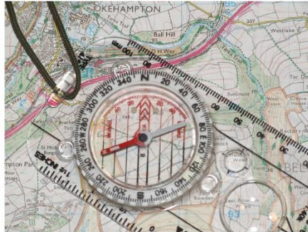
2: Rotate the compass housing so that it points to grid north
