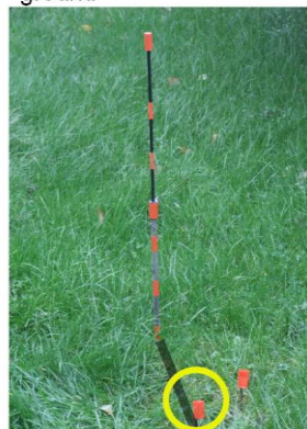
3. Wait 20 minutes and place the second marker at the end of the shadow which has moved
